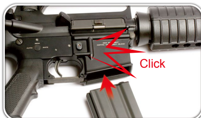
Insert the magazine into the body until you hear a 'click'.
